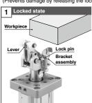
The lever is in the locked state when the lock pin is hooked on the bracket assembly.
