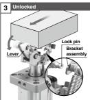
When the lock pin is unhooked from the bracket assembly, the lever becomes unlocked, which allows the workpiece to pass through.
