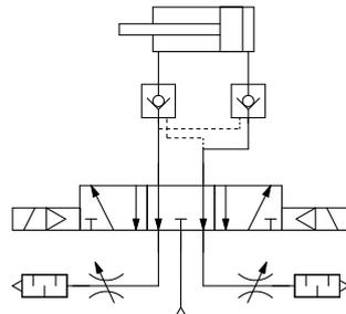
Residual pressure behind the exhaust needle may cause the pilot check valve to malfunction.
