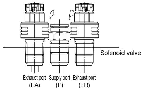
Fig. Example of the interference with fittings
