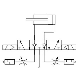
Residual pressure behind the exhaust needle may cause the check valve in the perfect valve to malfunction.
