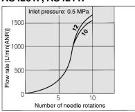
\* The numbers above the flow rate characteristics curves in the charts show the applicable tubing outside diameter as defined by the product number.
