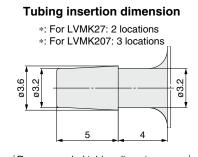
Recommended tubing diameter: I.D. ø2 to ø3.2, O.D. after mounting ø8 or less
