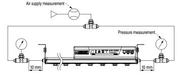
b) Air supply from both sides (Connecting tube: O.D.  $\emptyset$ 6 x l.D.  $\emptyset$ 4) (IZS4 $\square$ -820, 1120, 1300)
