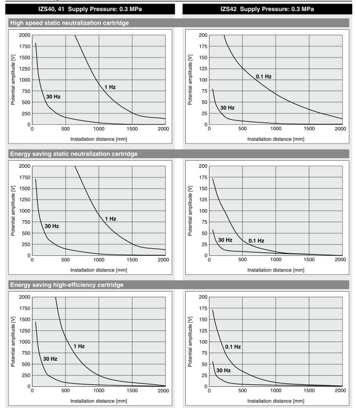
\* Static neutralization characteristics are based on data using a charged plate (Dimensions: 150 mm x 150 mm, Capacitance: 20 pF) as defined in the U.S. ANSI standards (ANSI/ESD STM3.1-2015). Use this data only as a guideline for model selection because the values vary depending on the material and/or size of the subject.
