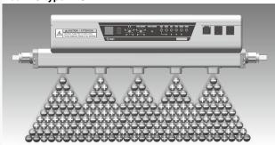
+ ions and - ions are discharged at the same time to allow the + and - ions to reach the workpiece evenly, thereby reducing the potential amplitude.
