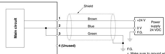
The cable colors shown in the diagram are for when the IZF10-CP power supply cable is used.
