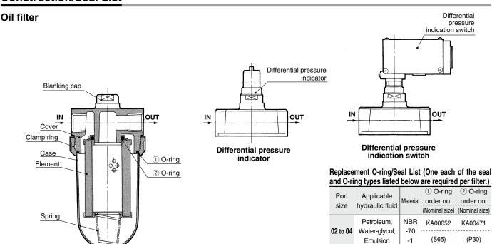
Note) The material and nominal size notations are based on JISB2401. (However, this doesn't include the nominal size of ① O-ring.)
